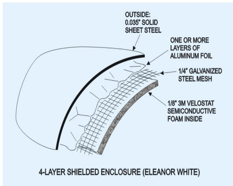
Seams were bolted and seams and corners stuffed full of compressed aluminum foil.
