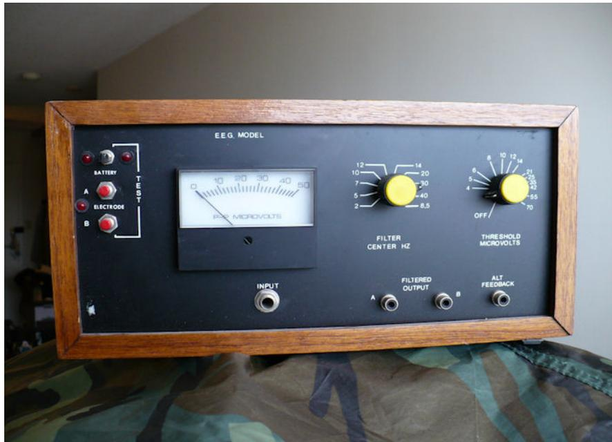
This biofeedback-style EEG unit does not have the paper strip chart seen on full-blown medical equipment. Instead it features two types of outputs: Meter reading, and geiger counter style clicks from its speaker. The more clicks, the higher the meter reading.
