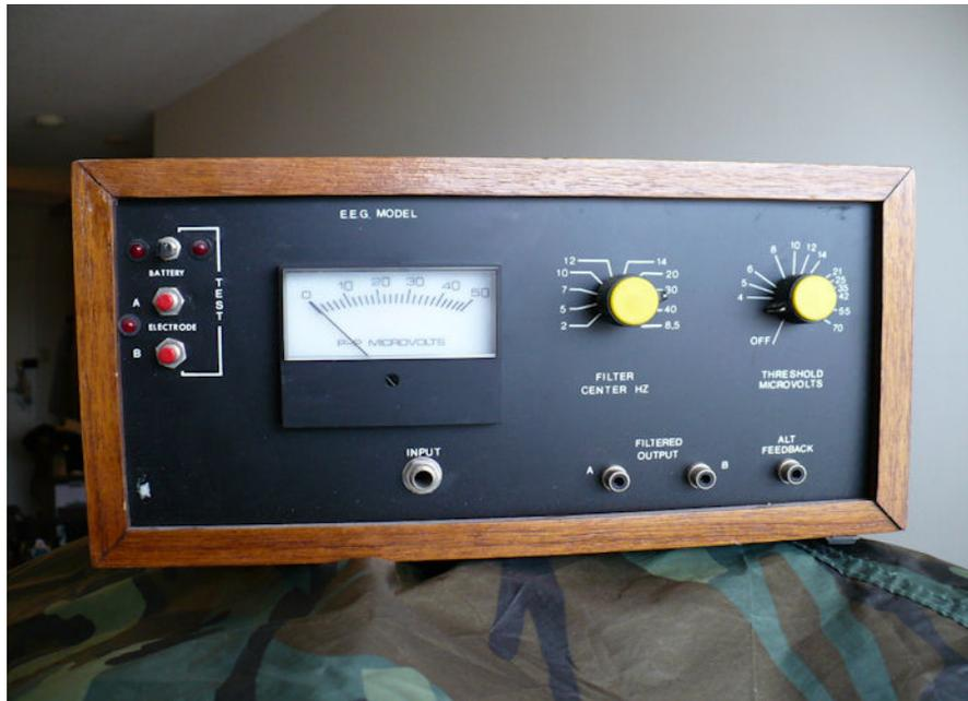
This biofeedback-style EEG unit does not have the paper strip chart seen on full-blown medical equipment. Instead it features two types of outputs: Meter reading, and geiger counter style clicks from its speaker. The more clicks, the higher the meter reading.
